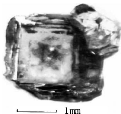
Figure 4. A diamond crystal grown using \text{Cu}_{43}\text{Co}_{57} for 20 h.
